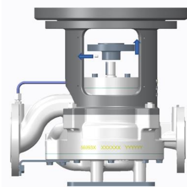
5. Loose Allen screw(34) ;Remove pump hub(33)
