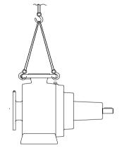
The lifting straps must not bear against sharp edges and corners.
